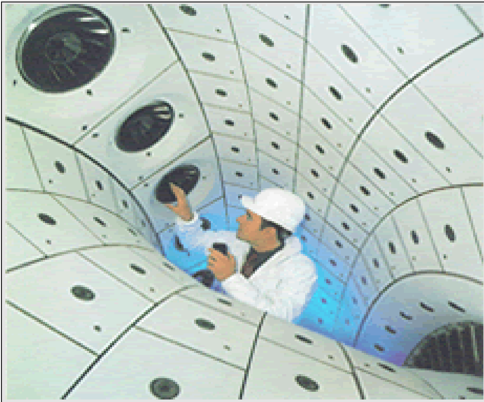
Siemens SGT5-4000F (V94.3A) Gas Turbine Combustion Chamber
