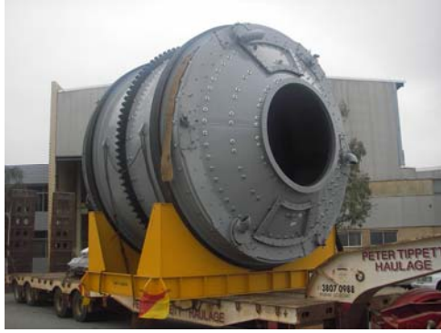
4.2m x 3.6m WEMCO HMS Drum Separator at BHP Mount Newman – iron ore separation.
