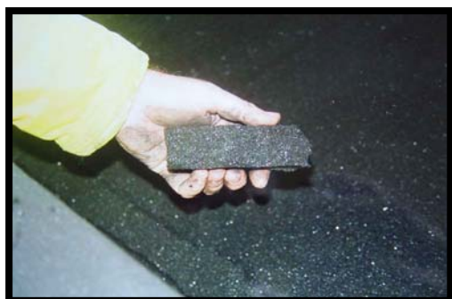
Tower filter Cake 4.6% Ash, 18.1% moisture.
